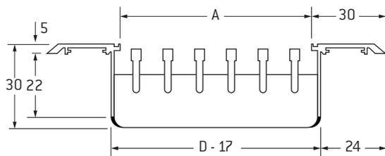
The same basic design as Model LD-1200 Linear Diffusers except that the Standard fixed, bar-type louvers are heavier 5.1mm x 16mm as compared to 3.2mm x 16mm.
