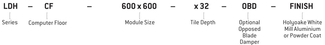
Holyoake LDH-CF Computer Floor supply grilles shall be of extruded aluminium, welded construction, with blades mechanically expanded into double, notched mullions spaced at nominal centres. They shall be designed to withstand a concentrated load of 500 kg over an area of 645mm<sup>2</sup> (1 square inch) at the centre, with no permanent distortion and maximum deflection under load of 0.66mm. Accessory volume control dampers, adjustable through the face, shall be furnished where indicated.
