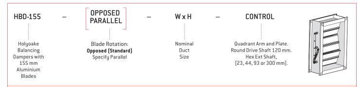
Balancing Dampers shall be of extruded aluminium construction. Frames shall be suitable for duct flange mounting. Blades shall be fixed to 11 mm hexagonal shafts held by two piece acetal self lubricating bearings, with outer shells fluted to prevent rotation.
