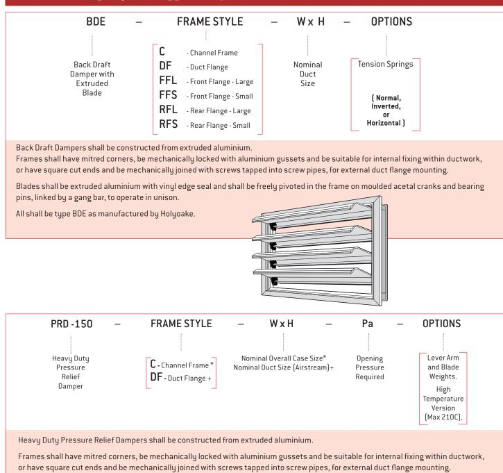
Blades shall be extruded aluminium with acetal edge seals both sides and be complete with aluminium side seal gaskets. They shall be linked by an aluminium gang bar, to operate together in unison. They shall freely pivot in the frame, on aluminium cranks and axles, within moulded acetal bearings. (Blade adjustment weights may be added if required, via a spindle control bar).
