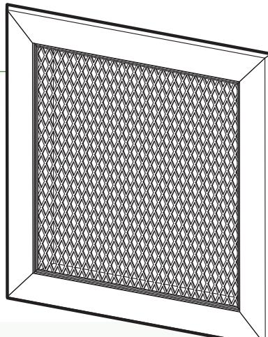
Return and/or exhaust Grilles shall be an aluminium frame with aluminium mesh core. They shall be of rattle-free construction, of the model shown on the drawings, or elsewhere in this specification. Frames shall have close mitred corners, reinforced and secured with aluminium gussets. Filter returns, where specified, shall be of similar construction, mounted in a hinged subframe and held closed with a positive latch. Filters are 'EU2' washable type.
