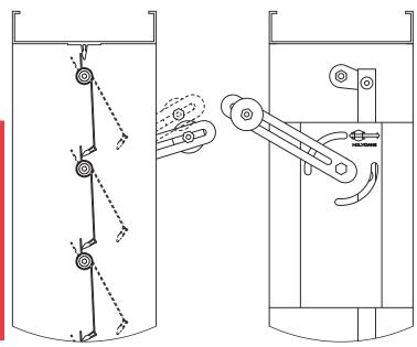
Factory calibration is not available; the correct amount of weight, with optional tension springs, is determined by on site commissioning by others.
